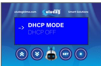
7 Press the UP button during 5 sec. to MENU-1. Find DHCP mode parameter from Menu by arrow buttons and do it DHCP OFF.
