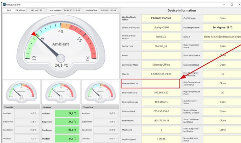
5 The static IP field appears empty. Double click here. This process will open the 4 lines below for information entry.
